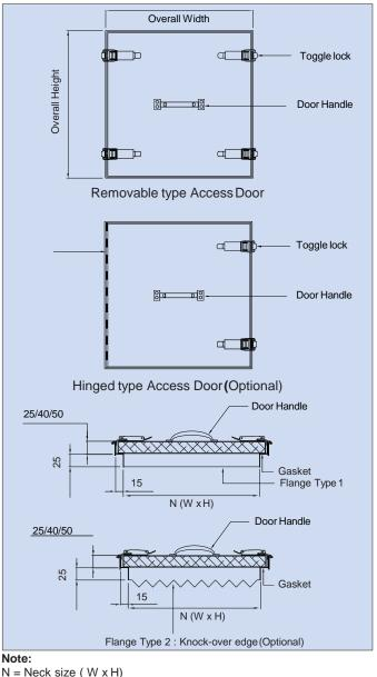
N = Neck size (W x H) Overall Width = Neck width + 30 mm Overall Height = Neck Height + 30 mm
